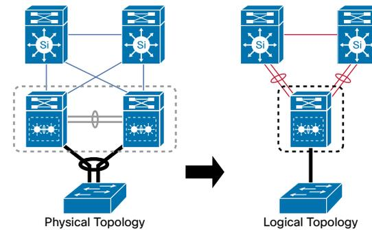
**Layer 3 Network Segmentation:** The traditional VRF-Lite solution usually requires a lot of configuration management. EVN reduces configuration time significantly across the entire network infrastructure without requiring the use of MPLS. Advantages include:
